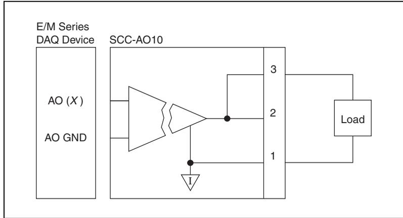
**Figure 1.** SCC-AO10 Connected to a Nonreferenced Load
