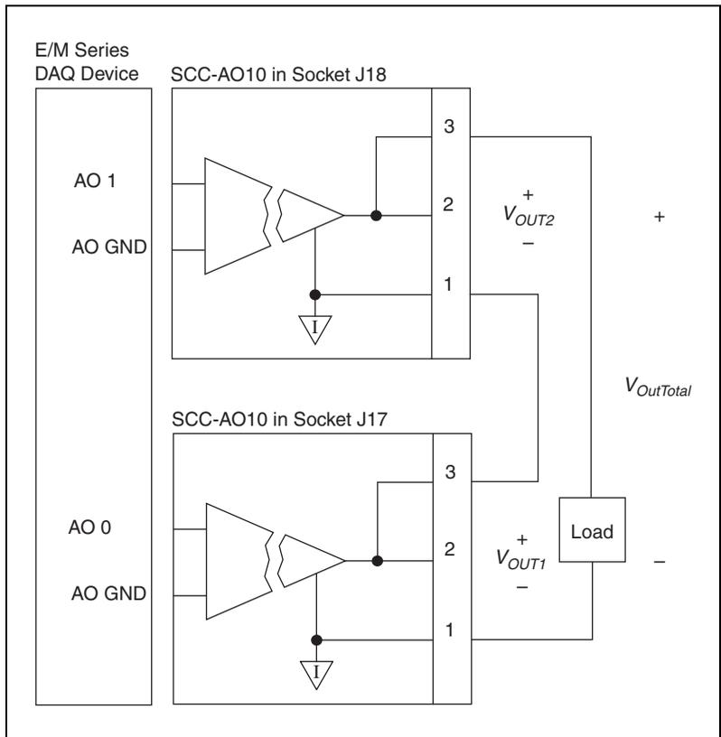
**Figure 3.** Connecting Two SCC-AO10 Modules in Series
