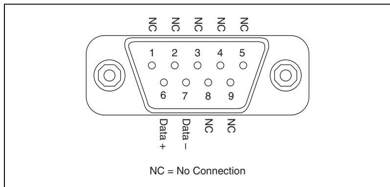
**Figure 2-6.** FBUS-HSE/H1 LD Connector Pinout
