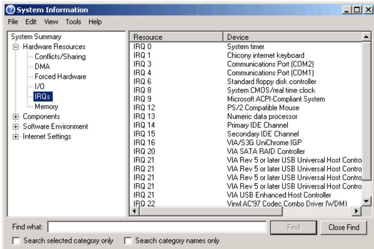
The MultiModemZPX only uses IRQs 3,4,and 5 so you need to check in the above screen to see if any of these IRQs are available. The MultiModemZPX is defaulted to IRQ 5.
