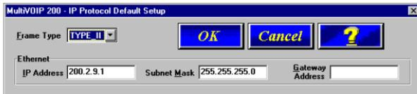
The default **Frame Type** is **TYPE\_II**. If this does not match your IP network, select the Frame Type from the **Frame Type** list. The Frame Type choices are **TYPE\_II** and **SNAP**.
