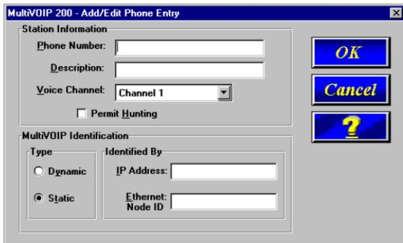
In the **Station Information** group, enter the unique phone number of the local device connected to Channel 1 in the **Phone Number** box. For example phone number 101.
