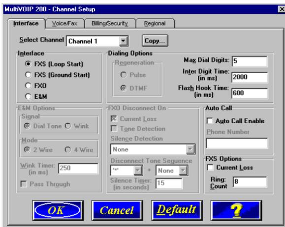
Configure each channel for the type of interface you are connecting to. To change the channel number, select the channel you want to configure from the **Select Channel** list.
