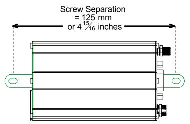
Drill the mounting holes at the desired mounting location (if applicable).
