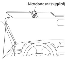
Secure the microphone cord using cord clamps (not supplied) if necessary.
