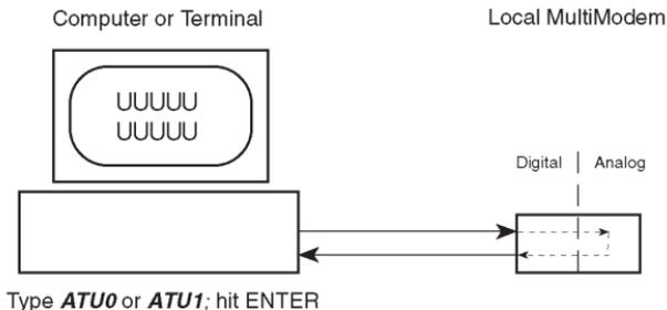
**Figure 6-1. Local Analog Loopback Test**
