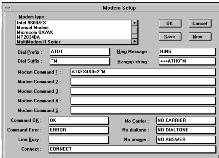
**Figure 3-1. The MEW Modem Initialization Setup**
