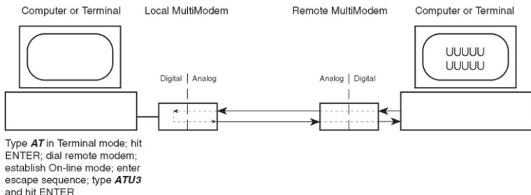
**Figure 6-2. Digital Loopback Test (local/manual)**
