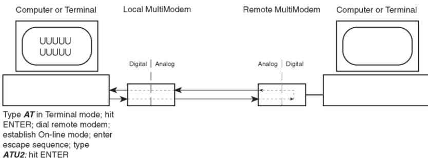
**Figure 6-3. Digital Loopback Test (remote/automatic)**
