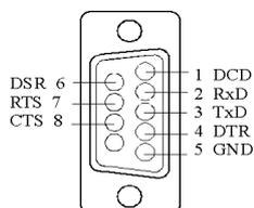
**Type 1: To connect the Industrio CP-114 Series to a DTE device.**
