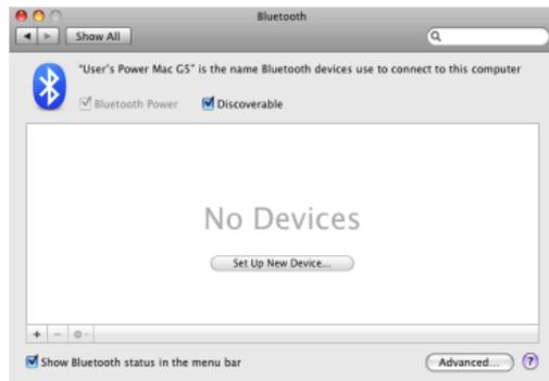
3. If you have already connected a device under 10.5 the Bluetooth window will look like this. Instead of clicking the Set Up New Device button, click the button with a plus (+) symbol below the device list.
