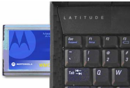
Figure 28. Installing the WMC6300 Wireless Modem Card
