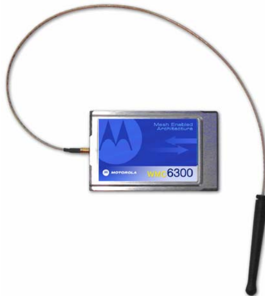
Figure 26. Attach the Antenna to the WMC6300
