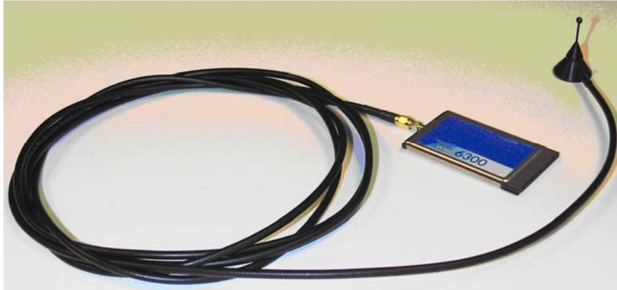
Figure 27. Attach Magnetic Mount Antenna to the WMC6300
