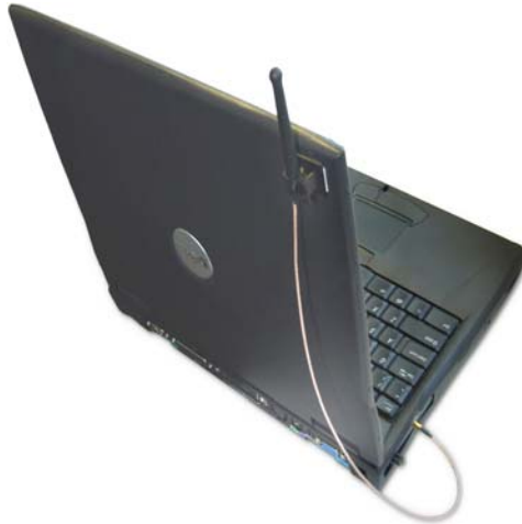
Figure 29. Proper Orientation of Antenna
