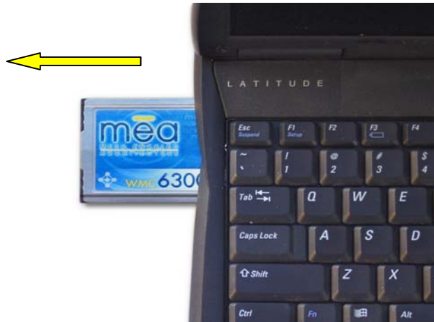
Figure 43. Removing the WMC6300 from the PCMCIA slot
