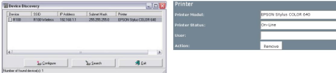
When properly setup, the R100 Wireless Gateway will show the printer name in the **Device Discovery** utility and show **On-Line** under the **Printer Server** on the **Status** page of the web manager.
