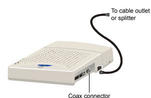
Allow 5 to 30 minutes to power up the first time because the Motorola Communications Gateway must find and lock on the appropriate channels for communications.
