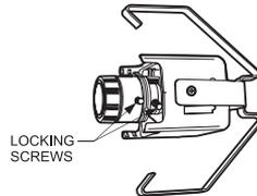
4. Always make sure the tab on the camera bracket is pointing out of the enclosure (away from the ceiling or wall). Gently squeeze the bracket, place it against the shoulder inside the base, and gently release.
