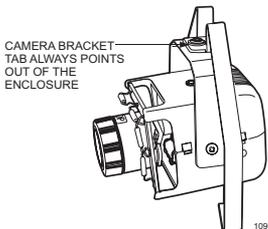
**Wall Mounting** – The camera bracket tab points out of the enclosure and the top of the camera points up towards the tab.
