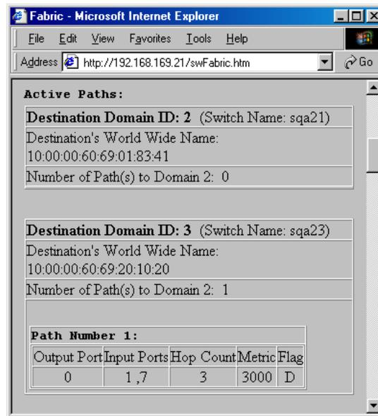
**Figure 3-5 Fabric Topology View, Scrolled Downwards**
