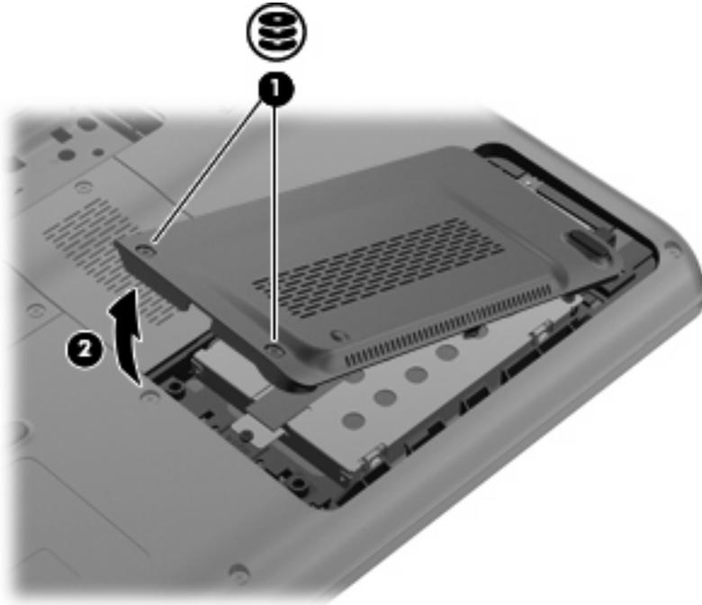
9. Remove the 3 hard drive screws.
