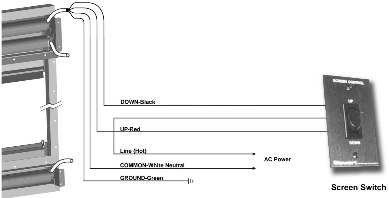
**Figure 9:** High voltage control wiring diagram
