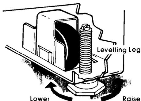
This refrigerator has 2 threaded levelling legs that are shipped in a separate package.
