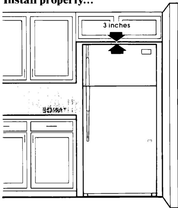
1. Allow 3 inches (7.5 cm) between overhead cabinets and the refrigerator top.
