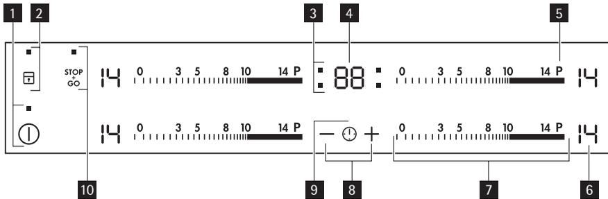
Use the sensor fields to operate the appliance. The displays, indicators and sounds tell which function operate.
