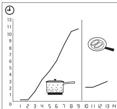
You can get a necessary heat setting in a shorter time if you activate the Automatic Heat Up function. This function sets the highest heat setting for some time (see the illustration), and then decreases to the necessary heat setting.
