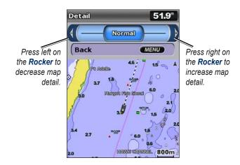
**Heading Line**—draws an extension line from the bow of the boat in the direction of travel
