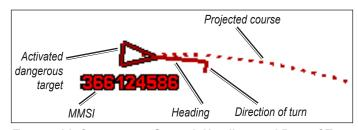
Target with Course over Ground, Heading, and Rate of Turn
