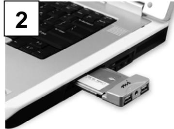
Carefully insert the PCMCIA Cardbus into an available Cardbus slot.
