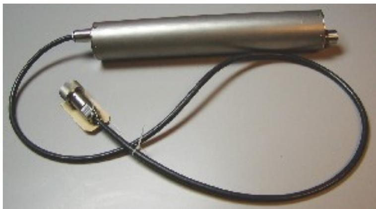
This form of DCM uses an integrated 26-pin connector to communicate, rather than having separate ports.
