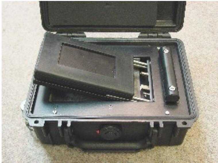
Slide the disk out and replace with another Lacie U&I drive, or any brand of IDE / USB or IEEE 1394 2.5" drive you specify (at the time of manufacture). You can do this at any time without losing data.
