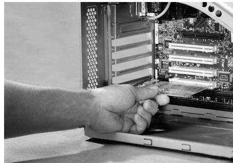
Figure 1 Installing the Adapter Card into a PCI Slot
