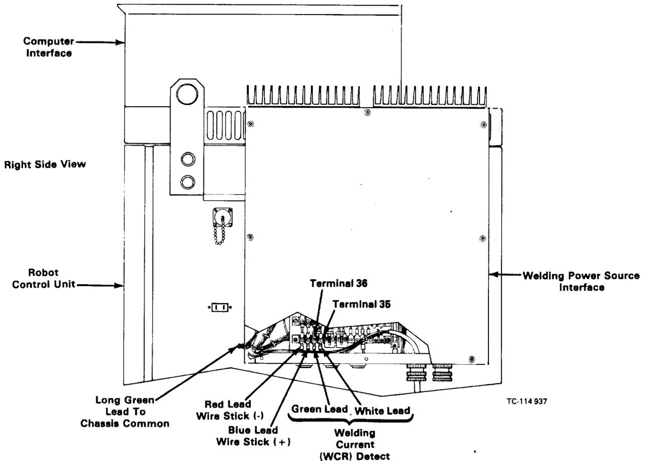
**Figure 2 - 3. Welding Power Source Interface Connections**
