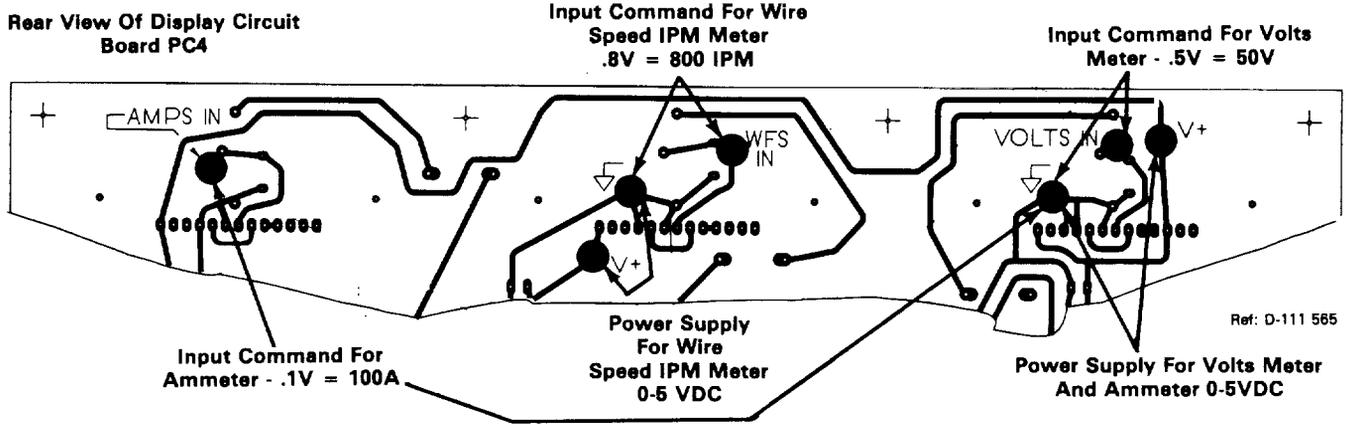
Figure 5 - 1. Display Board Meter Checks
