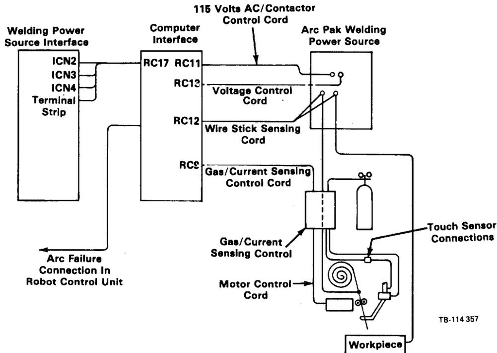
Figure 2 - 2. Interconnection Diagram
