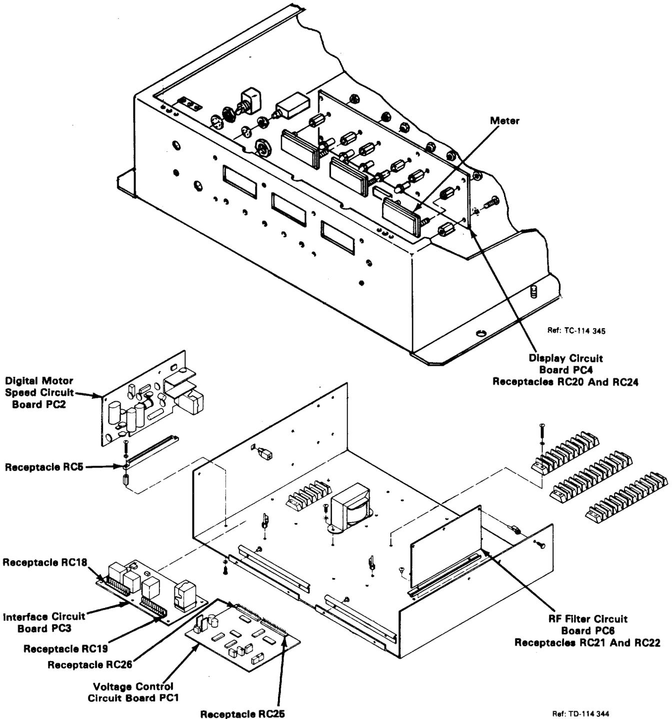
Figure 5 - 2. Circuit Board Replacement
