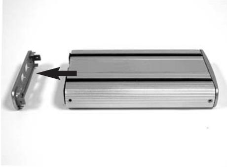
1. Remove the Back Panel from the Enclosure.
