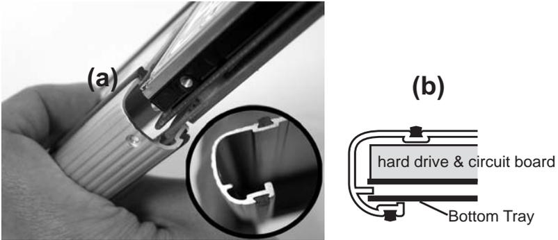
5. Align the Bottom Tray to the Sleeve Slot. Slide and push the hard drive/ Bottom Tray into the Enclosure Sleeve.
