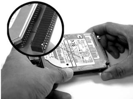
3. Align the pins on the hard drive to the 44-pin connector on the Circuit Board, and push the pins all the way in.
