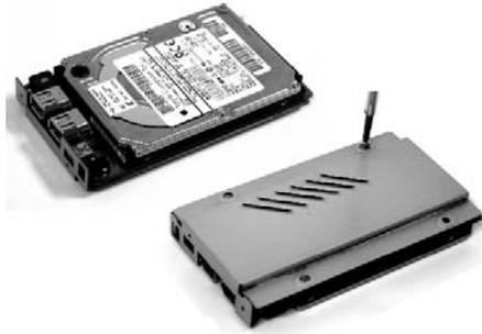
4. (a) Seat the Circuit Board and hard drive to the Bottom Tray. (b) Secure the hard drive with Screws (5mm in diameter) on the bottom of the tray.
