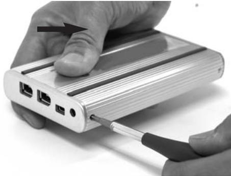
7. Secure the Back Panel with 2 screws (3mm in diameter) from each side.
