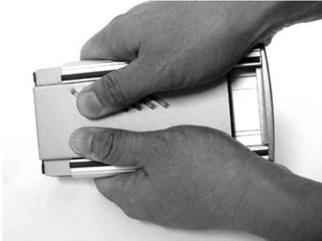
2. Use both thumb to push the Bottom Tray out.
