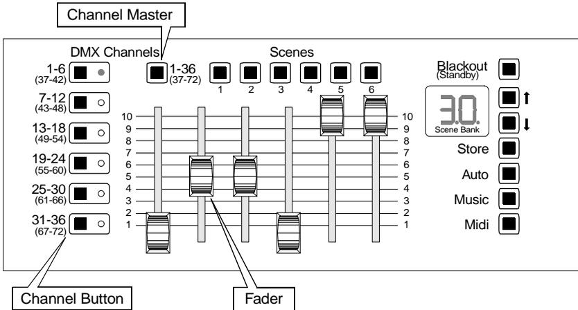
Lighting fixtures are controlled with the faders in groups of six channels. The DMX value is 0 when a fader is at the bottom and 255 when it is at the top. The faders map to the channels from left to right and can be calibrated using the procedure on page 24.
