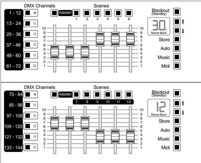
Two 2518 DMX Controllers with v. 2.1 or higher firmware and connected using the Tandem Connection Kit, P/N 91616005, can be operated in a 2-controller tandem mode in which DMX channels, faders, and scenes per bank are doubled.
