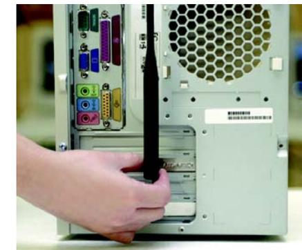
Figure 3-5: Positioning the Antenna
