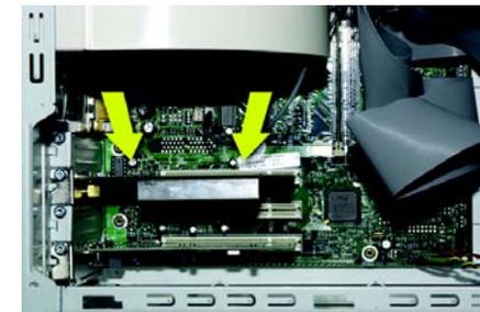
Figure 3-4: Installing the Adapter
