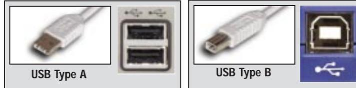
The **Type A** end connects to your computer's USB port. The **Type B** end connects to the Wireless USB Network Adapter.
