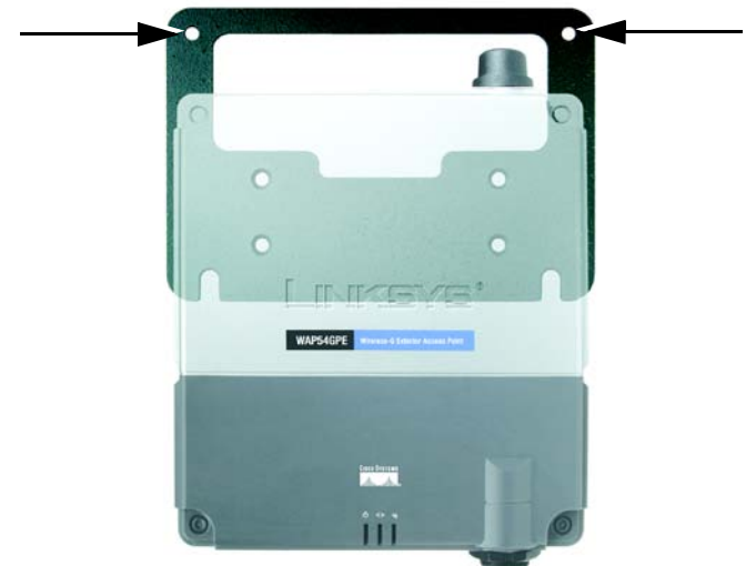
Figure 4-4: Attach the Access Point to the Wall
