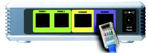
Figure 4-3: Connect to the Internet Port
