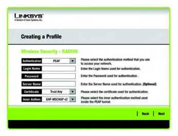
Figure 4-23: Wireless Security - RADIUS Using PEAP
