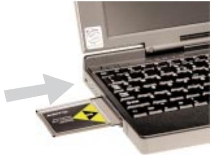
4. If your computer has more than one slot, insert the HomeLink Phoneline +10/100 Network PC Card into the first slot (slots are usually numbered in sequential order starting with 0 or 1). After verifying that the HomeLink Phoneline +10/100 Network PC Card's hardware and software are working correctly, you can always move the card to a different slot later if needed.
