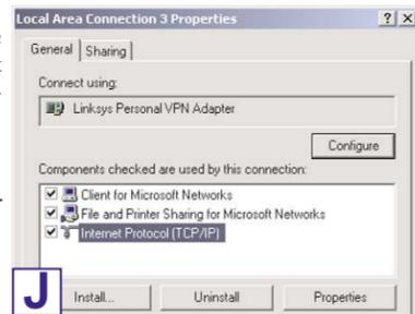
J. When the *Local Area Connection* screen is displayed, confirm that all of the following network components are installed:
