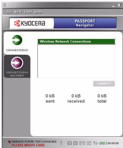
11. Insert your Passport PC card into your notebook's PC card slot with the label facing up. Raise the antenna so that it is fully extended and pointed up at a 90° angle. Use in any other configuration may exceed FCC RF exposure limits. Recognition of your card could take a few minutes while your computer recognizes the new software drivers that were installed in the previous steps.
