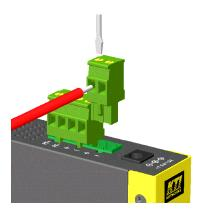
If cascading the power to next device is needed, install the power wires and plug for another switch. Then, use DC2 contacts.
