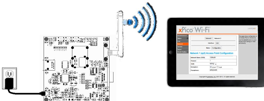
1. Once power and antenna is connected, turn on the board by moving switch SW3 in to the marked ON position.
