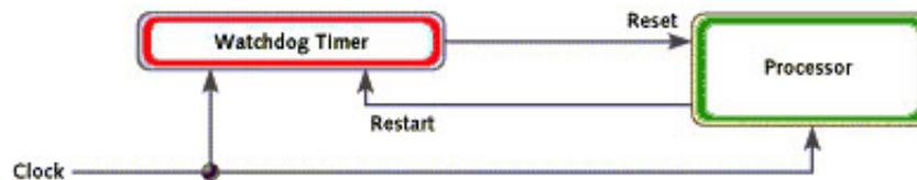
**Notes :** The watchdog function is design from the Intel 6300ESB. Lanner provide the sample code and Intel 6300ESB datasheet in the manual/driver CD. The path is under //WATCHDOG
