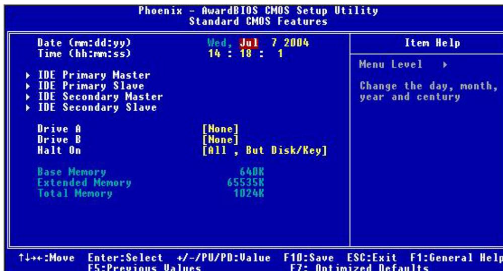
The Standard CMOS Setup utility is used to configure the following components such as date, time, hard disk drive, floppy drive, display and memory. Once a field is highlighted, on-line help information is displayed in the left bottom of the Menu screen.
