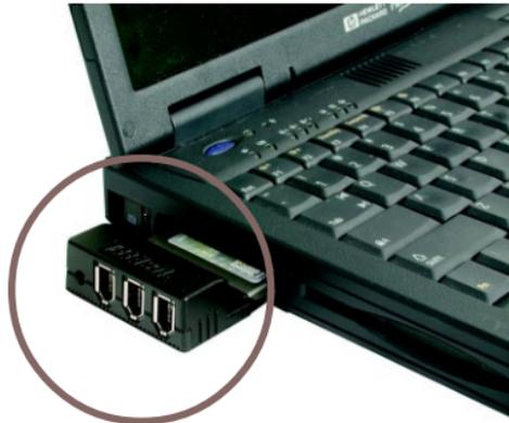
2. Start your notebook PC. If no Windows FireWire® driver is installed, then Windows will automatically detect the card and a dialogue box will appear, showing that the computer has located a **"PCI OHCI Compliant IEEE 1394 Host Controller"**. Windows will then prompt you for the location of the software driver. Then click **"Next"**
