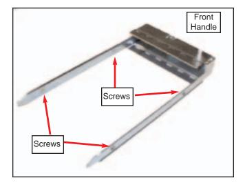
1. After removing the canister, place it on a static free surface along with the device to be installed.
