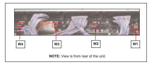
There are 4 jumpers on the personality card (W1, W2, W3, and W4) for hard setting the ID of each slot.
