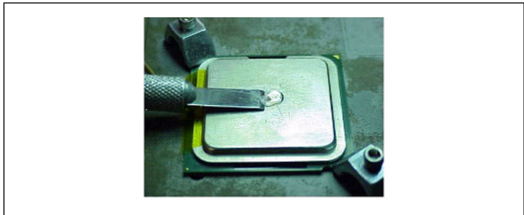
Figure 16. Removing Excess Adhesive from IHS
