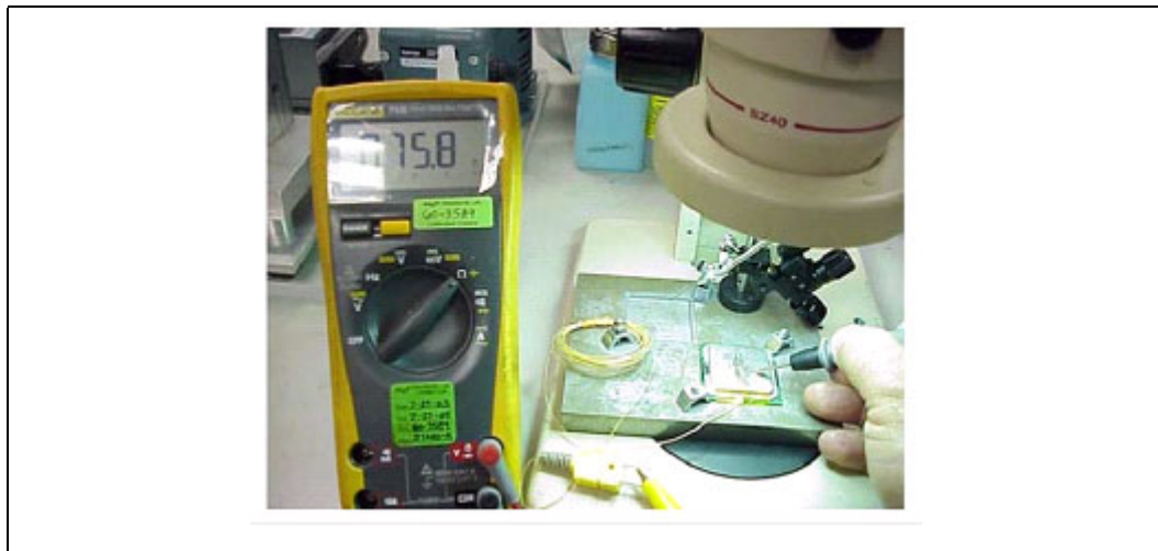
Figure 14. Applying Adhesive on Thermocouple Bead
