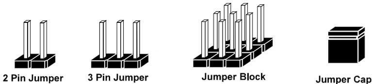
If a jumper has three pins (for examples, labelled PIN1, PIN2, and PIN3), You can connect PIN1 & PIN2 to create one setting and shorting. You can either connect PIN2 & PIN3 to create another setting. The same jumper diagrams are applied all through this manual. The figure below shows what the manual diagrams look and what they represent.
