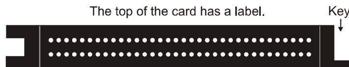
Figure 2. End view of the 50-pin PC-CARD connector showing proper orientation
