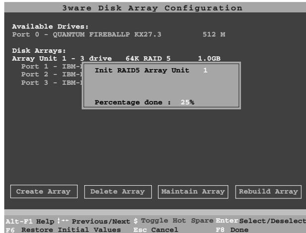
**Figure 10. BIOS Initialization Screen for RAID 5**
