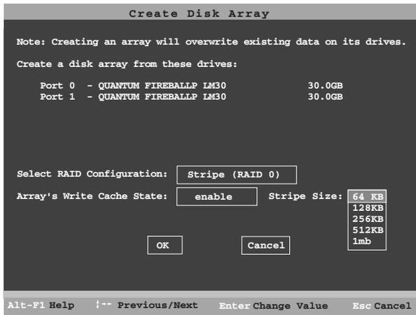
Figure 8. Create Disk Array Display, RAID 0 Example
