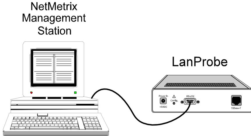
**Figure 3-15: LanProbe Direct Connection**
