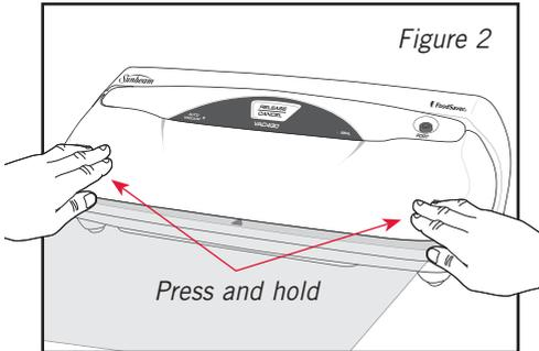
The motor will start. Continue to press and hold until the green auto-vacuum indicator light illuminates. See figure 3.
