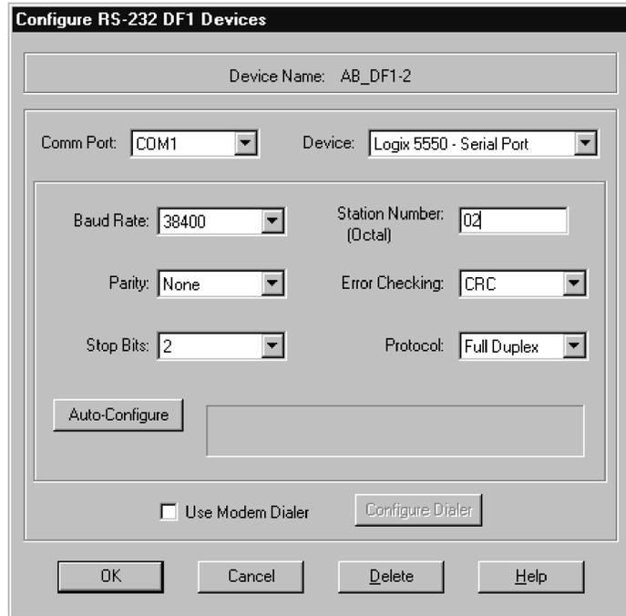
It is very important that the “Station Number” match the “Destn” number in ENI #1, assigned to the IP address for ENI #2. In this example, we arbitrarily used Destn address 2 to represent IP address 131.200.50.94, which is the IP address of ENI #2.
