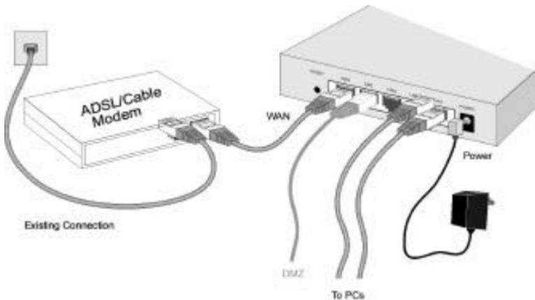
2. Use standard LAN cables to connect PCs to the LAN ports on the Soho 401 VPN.
