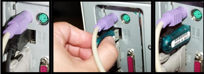
*Installation of the USB Key Block*
