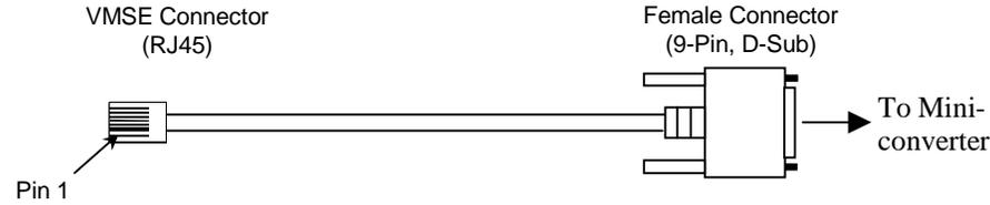
Figure 6-6. VMSE RJ45 Serial to RS232/485 Miniconverter
