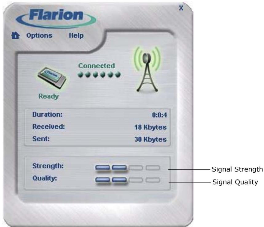
**Figure 14: Signal Strength and Quality Indicators**
